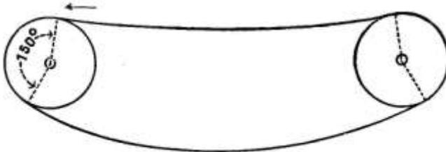
Showing Drive with slack side below and driving side above.
