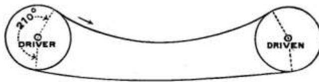
Showing Drive with slack side above and driving side below.
